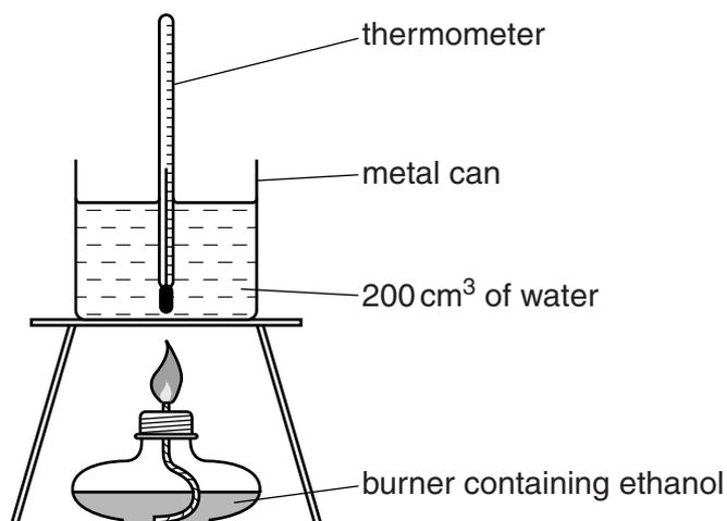
Some ethanol is put into the burner which is then weighed.
